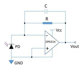
$$\begin{split} &V_{out}\left(V\right) = I_{ph}\left(A\right) \times R\left(\Omega\right) \\ &I_{ph}\left(A\right) = R_{\lambda}(A/W) \times A\left(cm^{2}\right) \times P\left(W/cm^{2}\right) \\ &\text{where A is chip area, P is incident UV power density} \\ &\text{and } R_{\lambda} \text{ is responsivity at specific wavelength.} \end{split}$$
